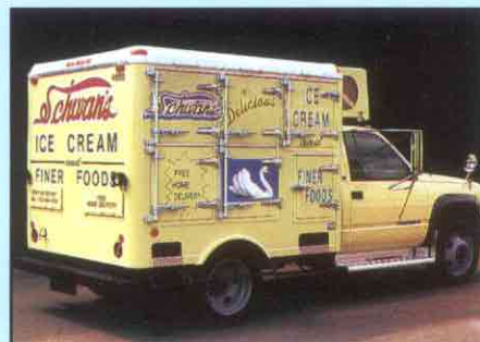
REFRIGERATED "REACH-IN" TRUCK BODIES FOR ICE CREAM DISTRIBUTION CAJAS REFRIGERADAS TIPO "REACH-IN" PARA DISTRIBUCION DE HELADO
