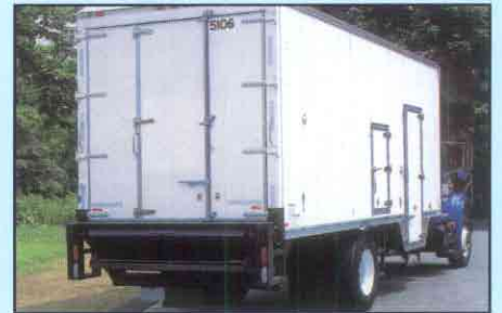
THERMALLY INSULATED TRUCK BODIES (7 TO 36 FT. LONG) WITH OR WITHOUT REFRIGERATION SYSTEM: FORCED AIR OR EUTECTIC PLATES CARROCERIAS CON AISLAMIENTO TERMICO PARA CAMIONES (7 A 36 PIES DE LARGO) CON O SIN SISTEMA DE REFRIGERACION: AIRE FORZADO O PLACAS EUTECTICAS
